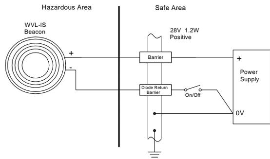
Fig 4 Single stage alarm using two channel barrier.
